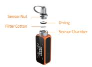
The filter cotton is used in the vacuum chamber to filter impurities and reduce sensor pollution. In order to maintain the best measurement accuracy, normal use needs to be checked every three months (adjust the inspection period according to the frequency of use). If the filter is seriously polluted, it needs to be replaced.
